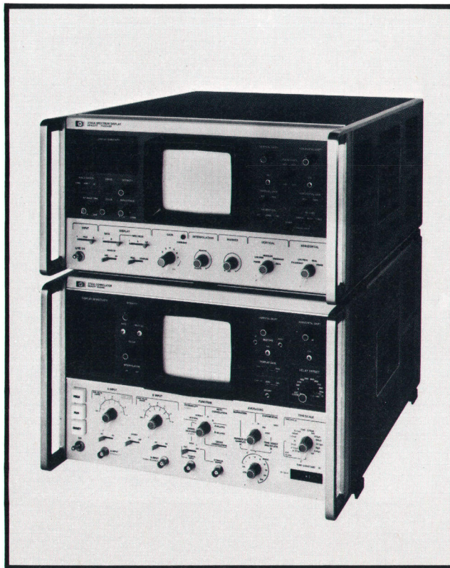
Fig. 1. New Model 3720A Spectrum Display (top) complements 3721A Correlator (bottom). Spectrum Display accepts correlation functions computed by Correlator and transforms them into the frequency domain, computing real and imaginary coefficients at 100 different frequencies.
